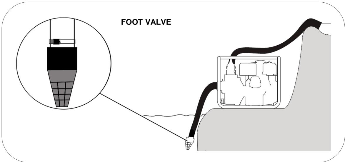
At first using the motor pump (**if using the foot valve**) completely fill the hose and pump body with water. The next times you use it will not be necessary to keep it always filled with water.
