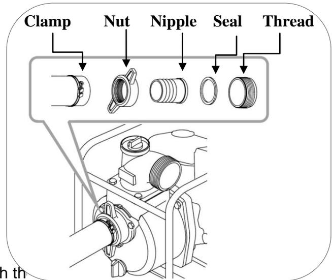
**The right connection of the intake hose is relevant for the correct water intake of the pump. Any small air intake between the connecting elements or in the hose itself would harm the water aspiration, especially if water is aspirated in depth.**
