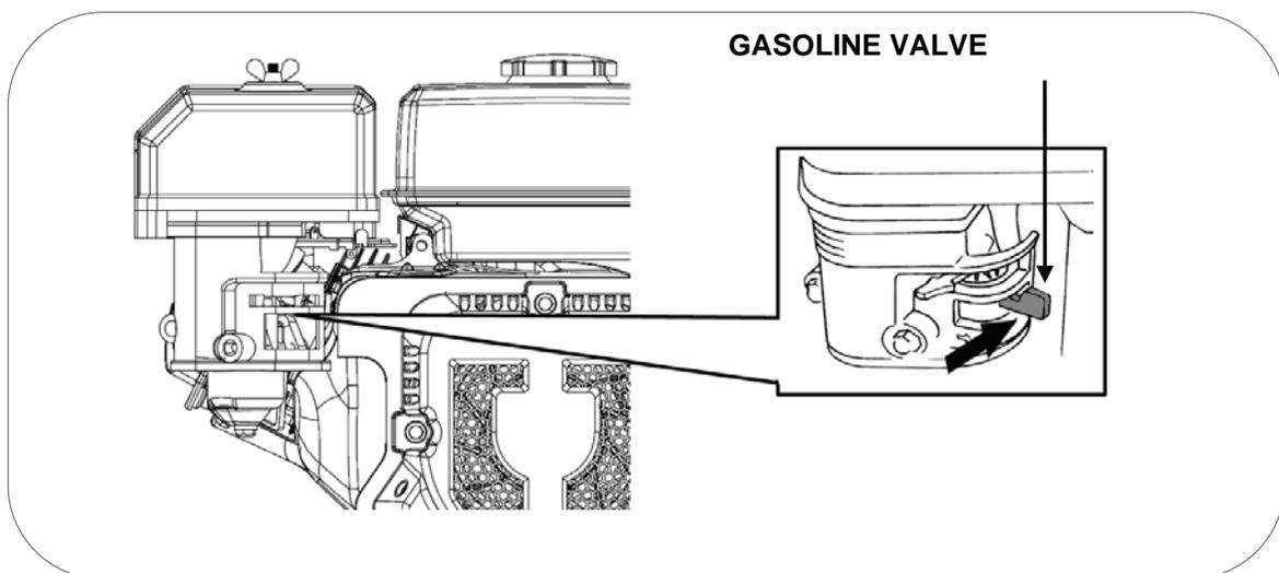
**IMPORTANT:**TAJO, NERVION and CANTABRICO models have an additional fuel valve at the outlet of the fuel tank, open turning upright, the other models with standard tanks do not have this valve.
