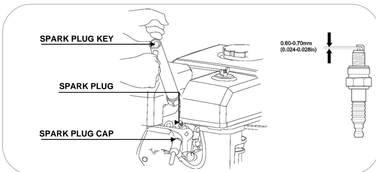
5 Measure the electrode distance with a gauge. Normal value 0.6 - 0.7 mm. Adjust the opening carefully if the value is not correct.
