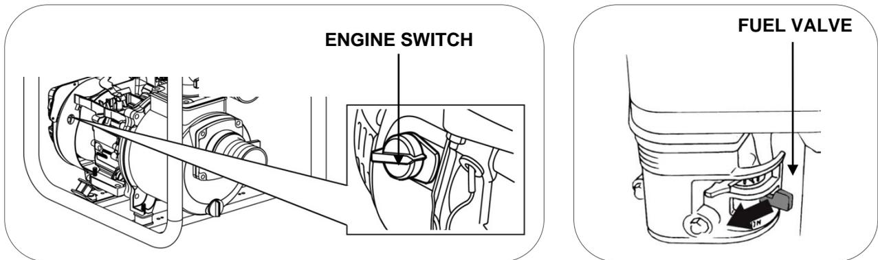
In **NERVION, TAJO, CANTABRICO** models close the gasoline secondary valve located at the outlet of the fuel tank, the other models do not have that valve.
