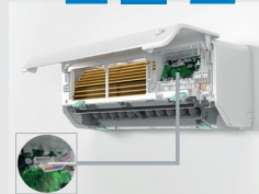
Open the electrical panel and disconnect the fan, louvers and ionizer motors
